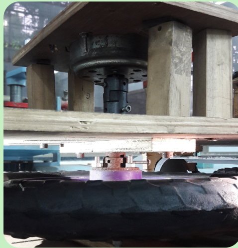
Shooting wheel and flex coupled motor
